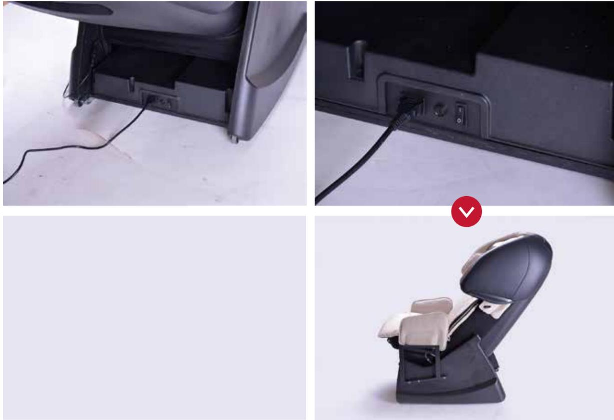
**4 Remove cotter pins and bolts from the chair base.** Locate the two cotter pins and bolts on the chair base. Locate the cotter pin and bolt on the link rod. Take them off and put them aside.
